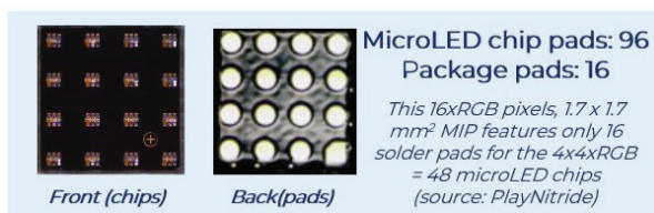
Fig. 8 reduction on the number and size increase of bonding pads with MIPs. Courtesy of PlayNitride
