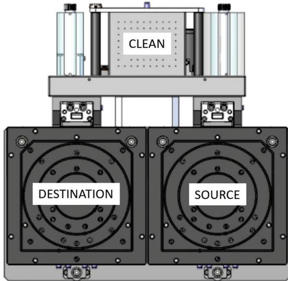
Fig. 4 Top view of substrate platen configured for up to 300 × 300 mm<sup>2</sup> source and target wafers and a roll-fed tape cleaning station.
