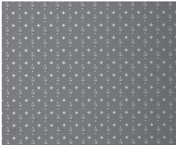
Fig. 5 Micrograph of the destination substrate populated with the microdevices at 423 PPI.
