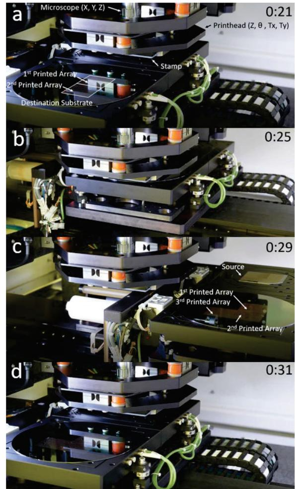
Fig. 6 Video captures from 10 s cycle mass transfer with a 750 × 750 device array stamp. (a) retrieval of the 3<sup>rd</sup> device array at 21 seconds. (b) alignment and transfer to the destination substrate at 25 seconds. (c) touch down onto the cleaning pad at 29 seconds. (d) device retrieval of the 4<sup>th</sup> array at 31 seconds.
