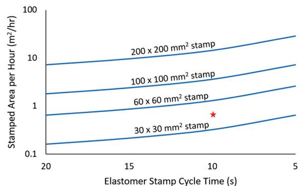
Fig. 7 Elastomer stamp transfer throughput depicted as the stamped area per hour for a single printhead versus the process cycle time. The red star represents the 10 second cycle time printing with the 750 × 750 array stamp.
