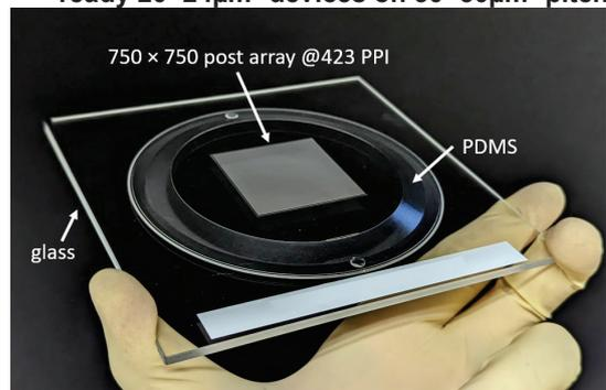
Fig. 2 Photograph of elastomer stamp that transfers a 750  $\times$  750 device array at 423 PPI.
