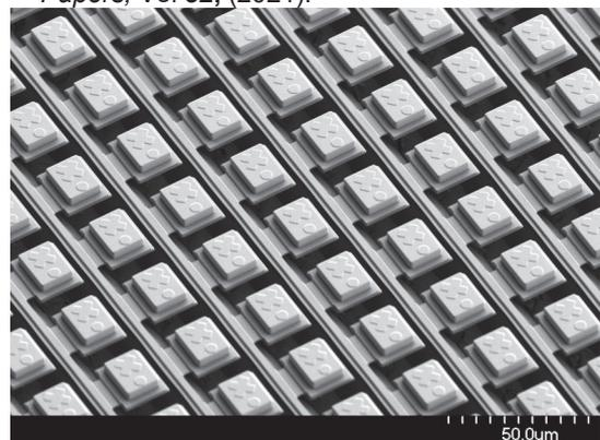
Fig. 1 Scanning electron micrograph of transfer-ready 20 $\times$ 24 $\mu\text{m}^2$  devices on 30 $\times$ 30 $\mu\text{m}^2$  pitch.
