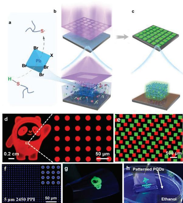
**Fig. 2** In situ direct photolithography fabrication of perovskite quantum dots pixels.
