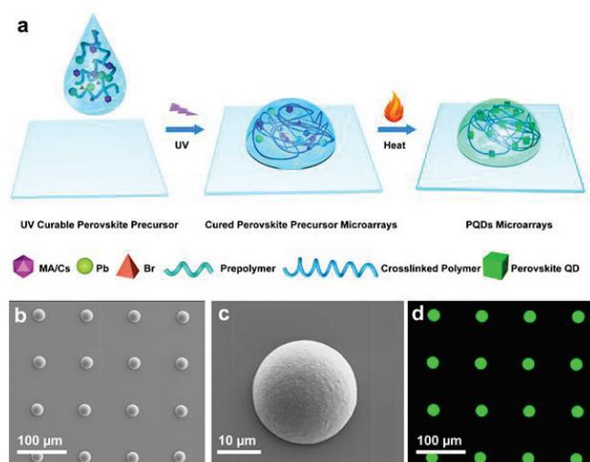
**Fig. 1** In situ direct print photopolymerization fabrication of perovskite quantum dots pixels.
