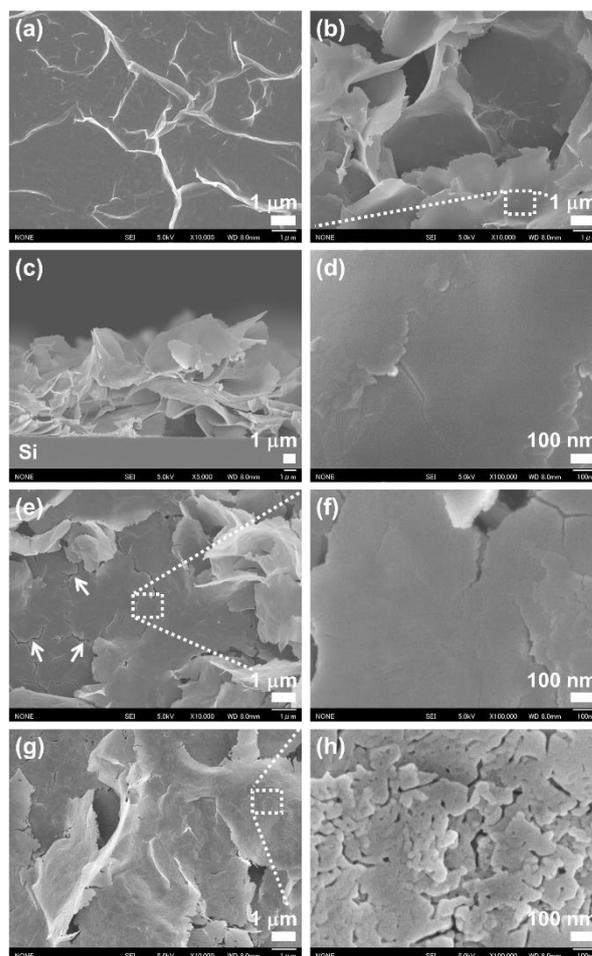
**Fig.3.** FESEM images of nanostructure samples with various growth times and annealing temperatures; (a) 2 h, without annealing treatment, (b-d) 6 h, without annealing treatment, (e,f) 6 h, with annealing at  $300\text{ }^\circ\text{C}$ , (g,h) 6 h, with annealing at  $500\text{ }^\circ\text{C}$ .
