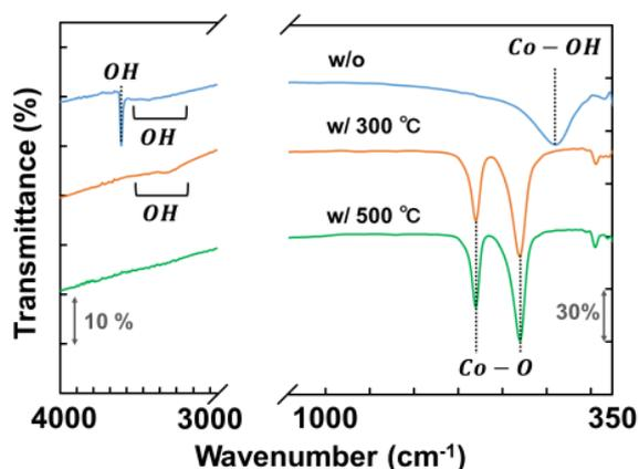
**Fig.2.** FTIR spectra of obtained samples with various annealing treatment temperatures; Growth time was 6 h.
