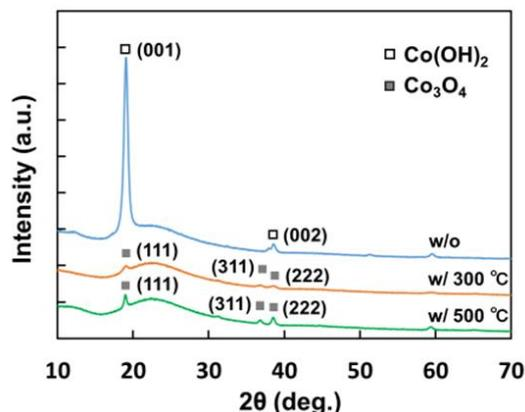
**Fig.1.** XRD patterns of obtained samples with various annealing treatment temperatures; Growth time was 6 h.
