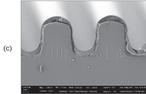
**Fig. 6 The Cross-section of UTE Structure on Trench Wafer: (a) Top, (b) Bottom, (c) Top & Bottom**
