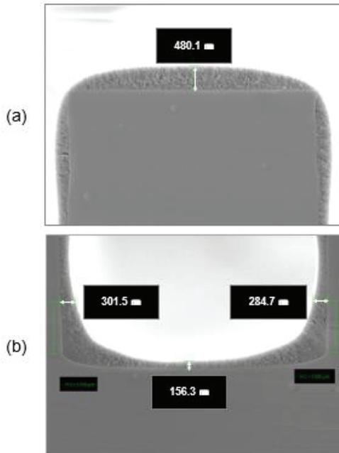
**Fig. 5 Trench Cross-section of iCVD Single Layer: (a) Top, (b) Side & Bottom**
