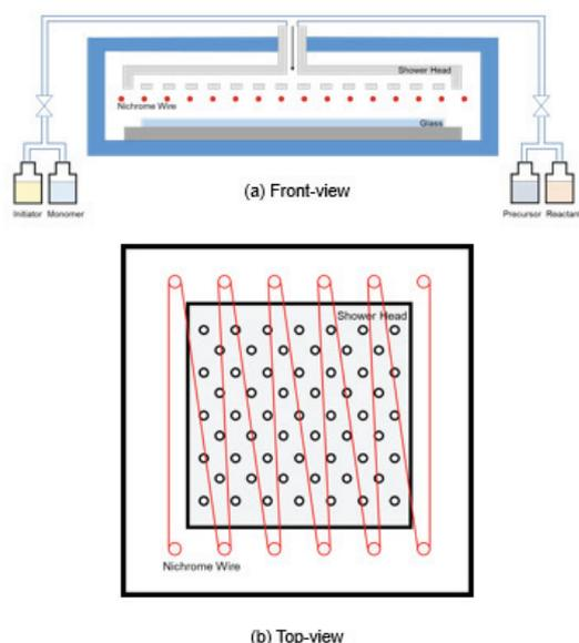
**Fig. 2 The Schematic of the iCVD and PEALD Hybrid System**
