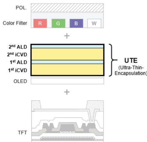
**Fig. 1 UTE(Ultra-Thin-Encapsulation) Structure**
