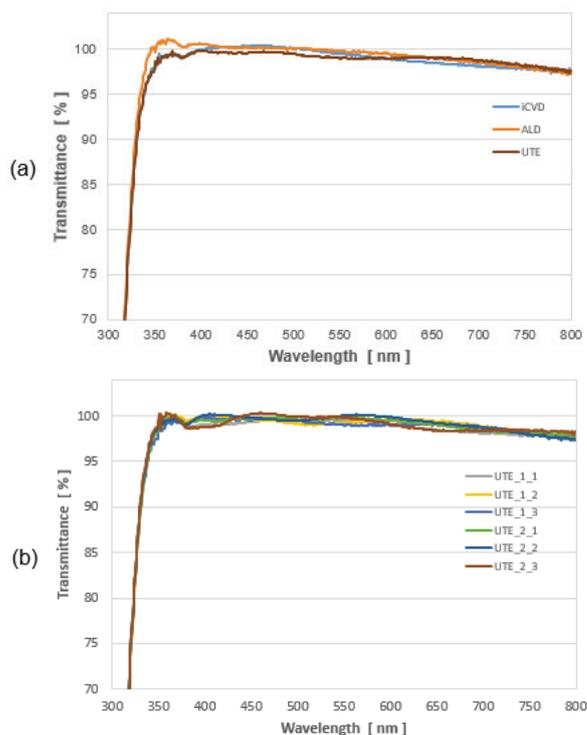
**Fig. 4 The Transmittance vs. Wavelength: (a) iCVD, PEALD and UTE Structure, (b) 6 UTE Structure Samples**
