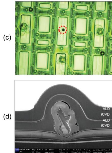
**Fig. 8 UTE Panel Fabrication: (a) On/Off test Jig, (b) 11-inch panel, (c) The dark spot in the 11-inch panel, (d) FIB image of the dark spot**
