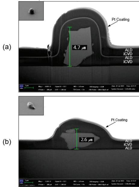
**Fig. 7 The FIB Cross-section: (a) UTE 2.0 Layers, (b) UTE 1.5**
