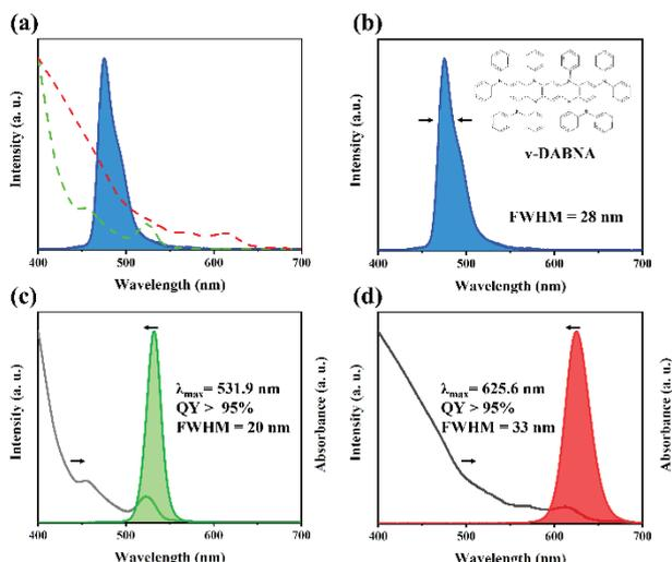
**Fig.1 (a)(b) Comparison of EL spectrum of v-DABNA as a hyperfluorescent material in blue OLED and absorbance spectra of GQD (green dash line) and RQD (red dash line), (c)(d) absorbance and photoluminescence spectra of GQD and RQD.**
