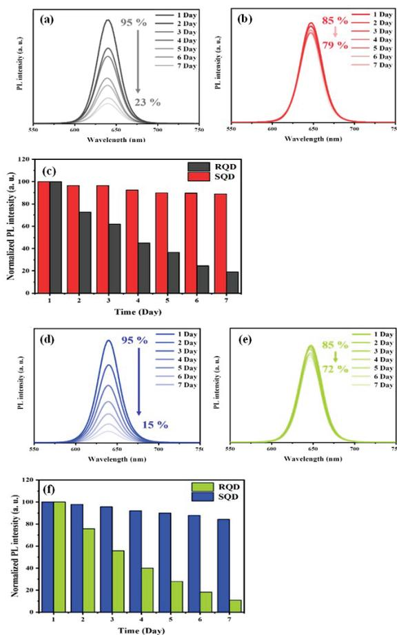
**Fig. 2 Comparison of PL intensity; initial and final PLQY of the (a)(d) (un-encapsulated) RQDs, (b)(e) siloxane-encapsulate RQD. Histograms - changes in relative PL intensity of each QDs (c)(f). Data (a-c) for thermal annealing at 120°C, and UV-irradiation (d-f)**
