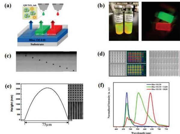
**Fig. 3 (a) Schematic illustration of QD CCL/blue OLED (b) photographs of QD solutions (c) Flight of ink droplet of RQD in a jetting cycle (d) Inkjet-printed pixels of GQD/RQD in the pixel-defining insulated layer (e) Printed pattern; RQD/TiO<sub>2</sub>/acrylic resin with > 3µm thickness dot/line pattern (f) Color conversion spectrum of GQD/RQD with blue OLED (0.14, 0.18) light source.**
