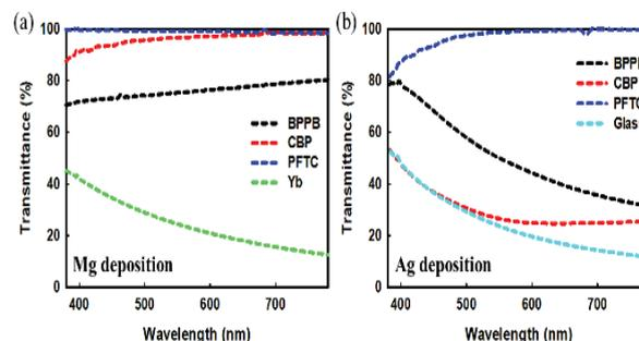
**Figure 2.** Measured transmittance of (a) Mg (b) Ag deposited cathode unit film on MPL materials.
