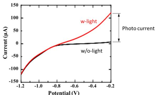
**Fig. 5 Photoelectrochemical measurement of QDs**
