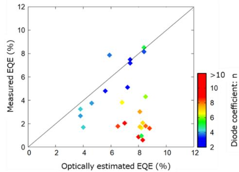
**Fig. 3 Measured and optically estimated EQEs with diode coefficients**
