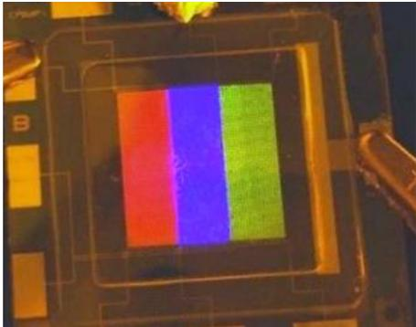
**Fig. 2 Electroluminescence image of RGB Cd-free QD-LED**
