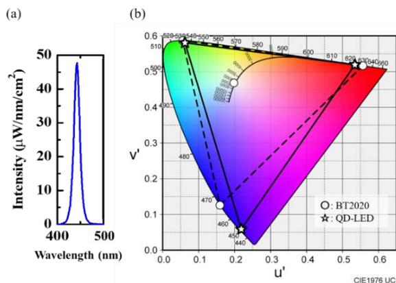
Fig. 1 (a) PL spectrum of Cd-free blue QD (b) Color gamut of developed QD-LED
