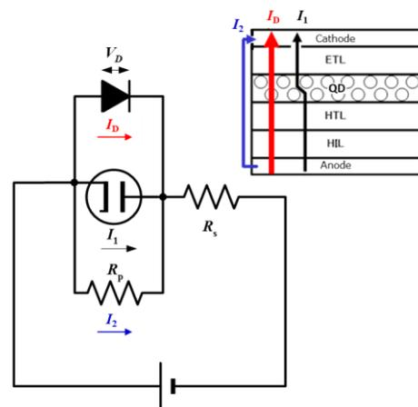
**Fig. 4 Equivalent circuit of QD-LED**
