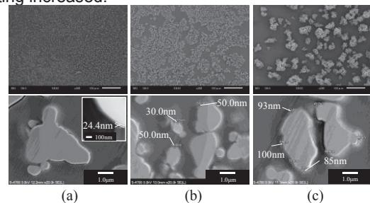
**Fig. 5 Top-view (upper) and cross-sectional SEM (lower) images of SrGa<sub>2</sub>S<sub>4</sub>:Eu particles with (a) thin coating (b) medium-thickness coating and (c) thick coating**
