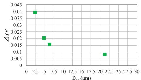
**Fig. 4 Particle size dependence of chromaticity change Δu'v' during aging for uncoated SrGa<sub>2</sub>S<sub>4</sub>:Eu phosphors**
