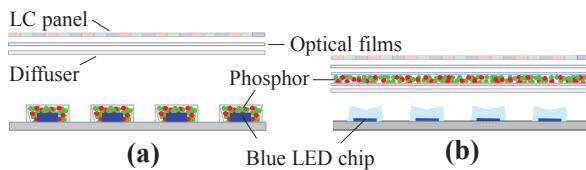
**Fig. 1 Typical schematics of a conventional BLU and a BLU using a phosphor film**
