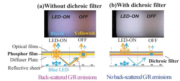
**Fig. 2 Schematic diagrams of blue emissions from blue LEDs and green and red emissions converted by phosphors in direct-type BLU with phosphor film implementing local dimming (a) without dichroic filter and (b) with dichroic filter**
