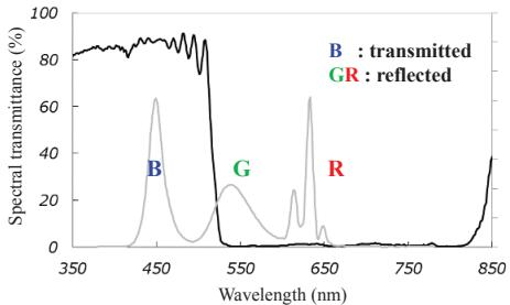
**Fig. 3 Spectral transmittance of dichroic filter**
