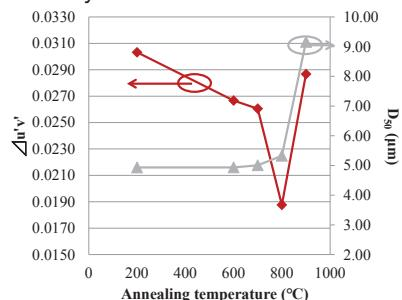
**Fig. 6 Particle size for SrGa<sub>2</sub>S<sub>4</sub>:Eu phosphors and chromaticity change  $\Delta u'v'$  during aging as function of annealing temperature**
