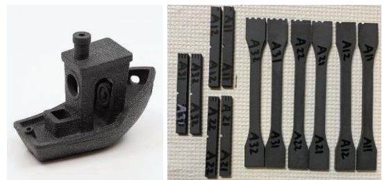
Fig. 5 Printed component (l.) and test samples for lab tests (printed with different orientations in powder bed; r.)
