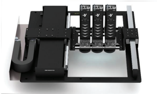
Fig. 1 AM subsystem with multiple projectors stacked in 1-axis motion system
