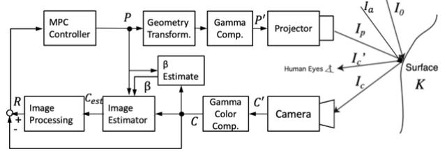
Fig. 4 AC with reflectance estimation compensation
