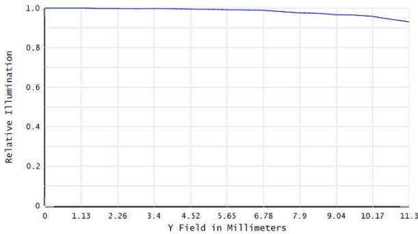
**Fig.5 The relative lamination of the lens group**
