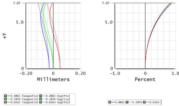
**Fig.4 Field curvature and distortion of this system**
