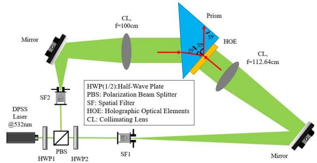
**Fig.7 The experimental structure of recording HOE**
