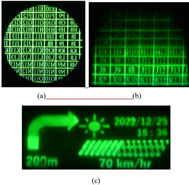
**Fig.9 (a) Image only pass through projection lens (b) Image from output HOE with eye relief of 300mm (c) Image from output HOE with eye relief 300mm and suitable size pattern**
