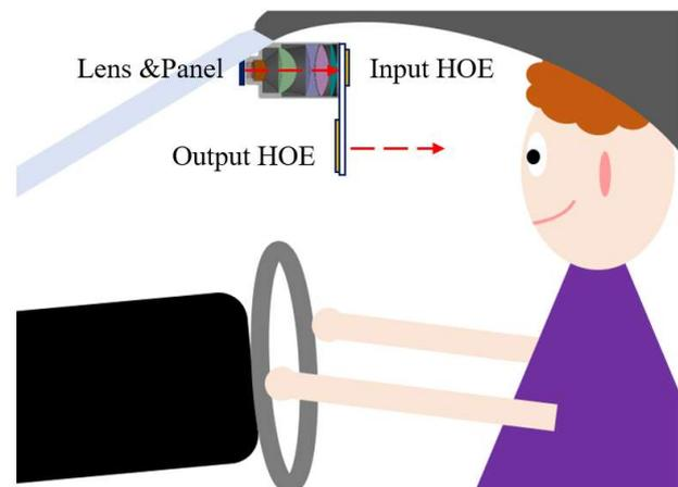
Fig.1 The schematic diagram of the location of the HUD in the car
