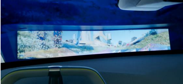
Fig. 11 Full immersive mode with tinted front screen
