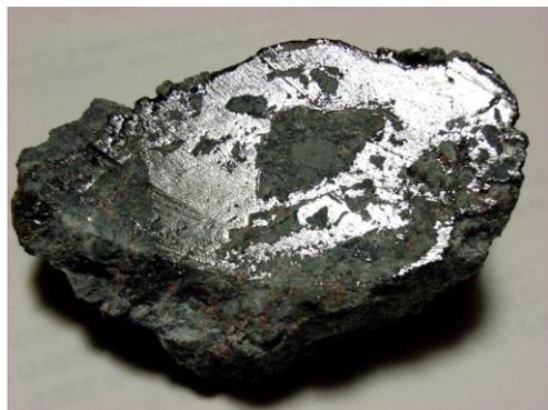
Arsenic: showing metallic luster by cutting (55mm width).
