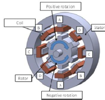
FIGURE 2. 8-6 type SRM structure
