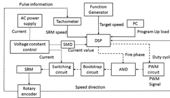
FIGURE 6. System flow of SRM drive system
