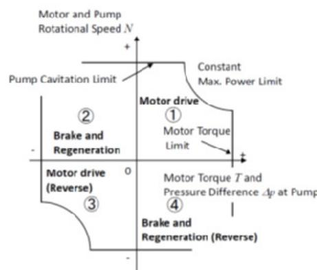
FIGURE 4. Operation range of hydraulic pump driven by servomotor
