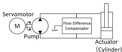
**FIGURE 1.** Valveless control system for hydraulic actuator drive (Closed circuit)
