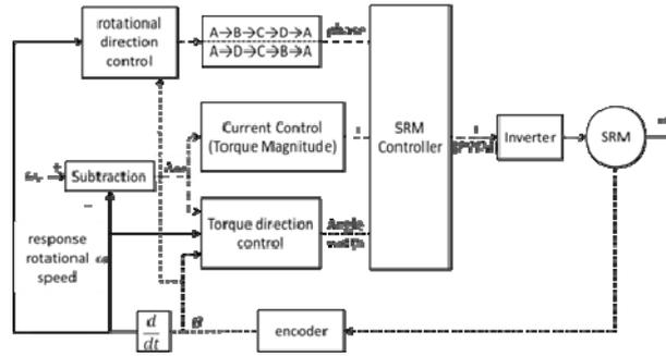
FIGURE 5. Bi-direction rotational speed control system of SRM
