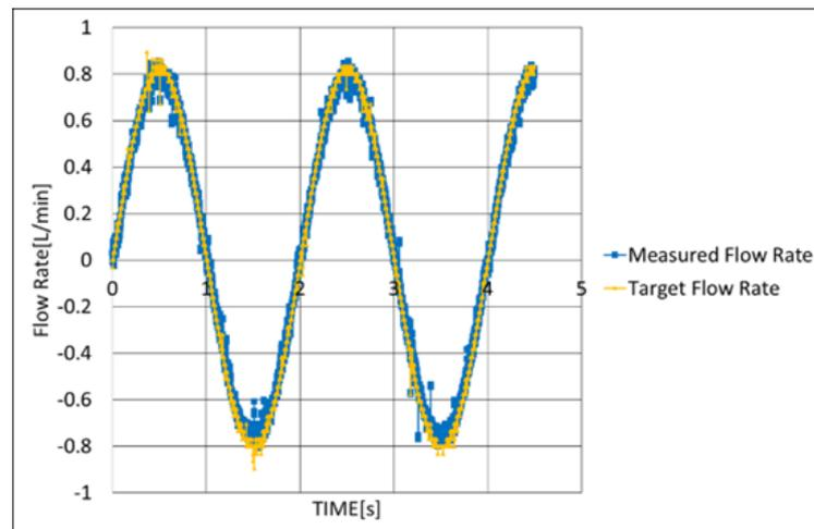
**FIGURE 8.** Sinusoidal bi-direction flow rate control of hydraulic pump driven by SR servomotor (SRM speed -1000rpm ~ +1000rpm)
