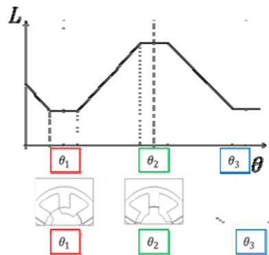
FIGURE 3. Conceptual self-inductance distribution between aligned and unaligned position
