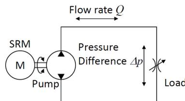
FIGURE 7. Testing hydraulic closed circuit for bi-directional flow rate control using hydraulic servo pump driven by SR servomotor
