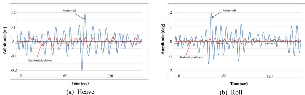
FIGURE 6. Measured heave and roll motions of the main hull and top plate
