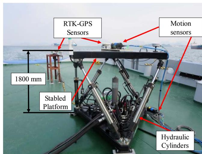
FIGURE 5. Scale model of the active vibration compensation system on the ship
