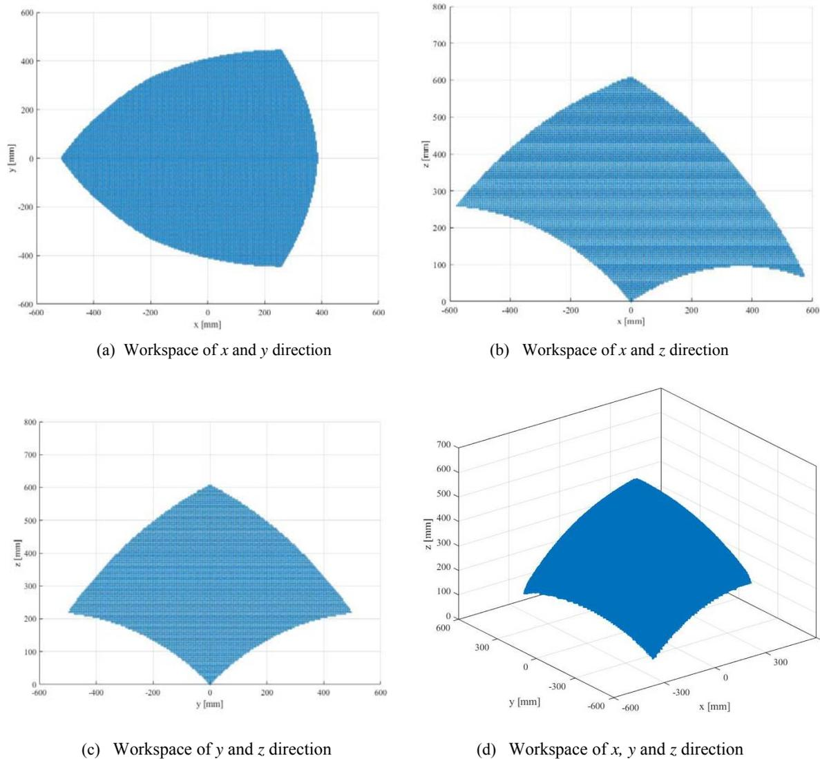
**FIGURE 8.** Workspace of the prototype of the parallel mechanism
