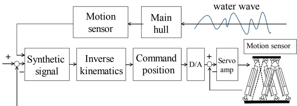
FIGURE 2. Configuration of the active vibration compensation system
