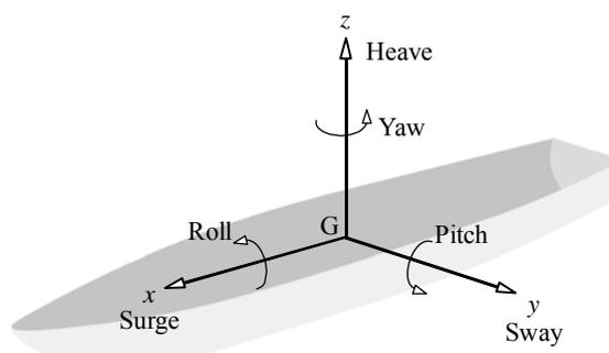
FIGURE 1. Six degrees of freedom for ship motion
