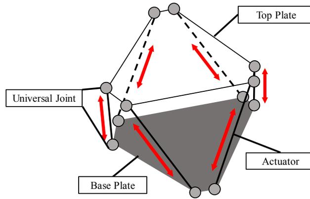
FIGURE 3. Stewart Platform type of parallel kinematic mechanism
