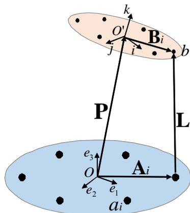
FIGURE 4. Vector diagram of parallel kinematic mechanism
