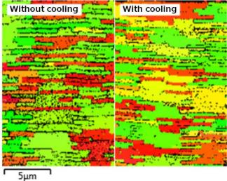
Fig. 2 EBSD maps of abalone nacre layers. (Acc. 5 kV, P.C. 5.7 nA, S.S. 100 nm, Without noise reduction) Black points in maps are index errors.
