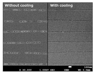
Fig. 1 FE-SEM images of an abalone nacre layers. Samples are processed by Ar ion beam with and without cooling.
