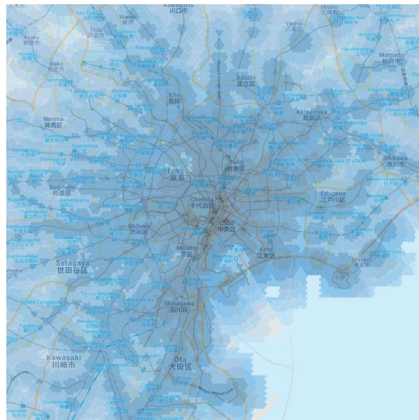
Figure 1. Isochrone map of Tokyo centered on Tokyo Station using the train+walk network. Darker colors indicate shorter travel times.
