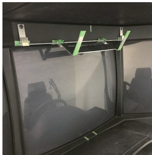
Fig. 5 Experimental setup of Kinect on Driving simulator
