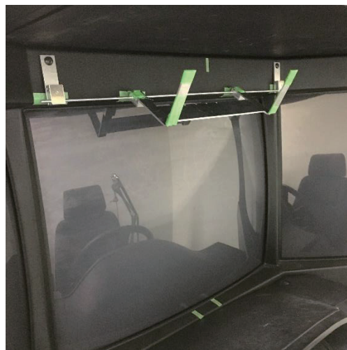
Fig. 5 Experimental setup of Kinect on Driving simulator
