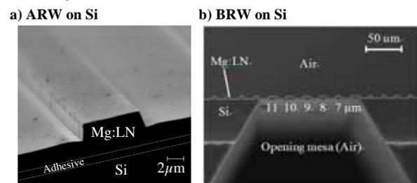
Fig.2 Mg:LN ridge waveguide on Si platform:
