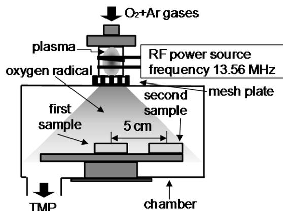
Fig.1: Schematic apparatus for oxygen radical treatment.
