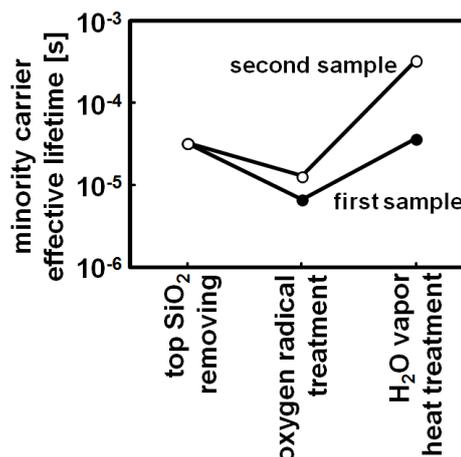
Fig.2:  $\tau_{\text{eff}}$  for samples in the cases of top SiO<sub>2</sub> removing, oxygen radical treatment, and 1.3x10<sup>6</sup> Pa H<sub>2</sub>O vapor heat treatment.
