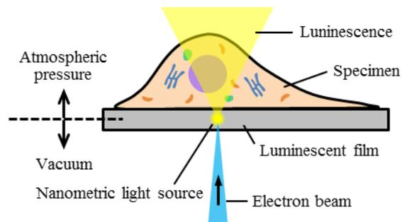
Figure 1: schematic diagrams of focal point in the EXA microscope. In this study, the luminescent film is  $\text{Si}_3\text{N}_4$  thin film or  $\text{Si}_3\text{N}_4 + \text{Y}_2\text{O}_3:\text{Eu}$  thin film.
