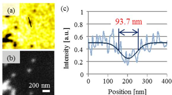
Figure 2: (a) Observation result of  $98.8 \pm 7.9$  nm gold nanoparticles with the EXA microscope. (b) A back scattered electron image of gold nanoparticles with a SEM. The Scale bar is 200 nm. (c) A line profile of the line in (a).
