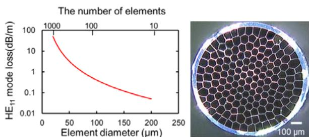
Figure 1. Calculated  $HE_{11}$  mode loss (left) of fiber bundles and a micrograph of a fabricated fiber bundle (right).
