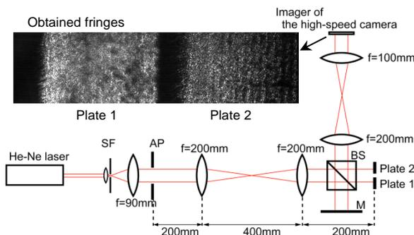
Fig. 1. Optical configuration for interferometric vibration analysis.
