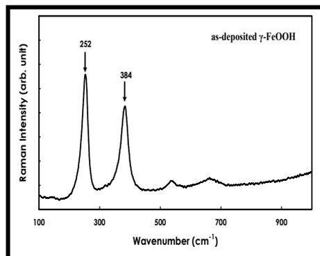
Fig. 1 Raman shift of the as-deposited  $\gamma$ -FeOOH thin film.
