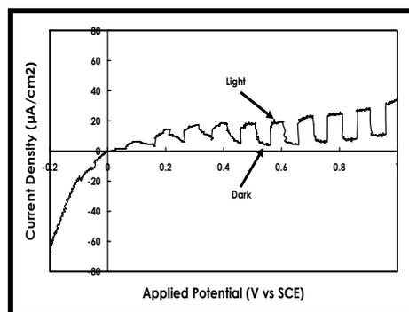
Fig. 3. Photosensitivity of  $\gamma$ -FeOOH film.
