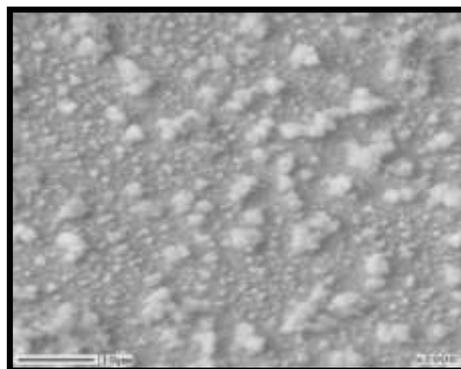
Fig. 2. SEM photograph of the as-prepared  $\gamma$ -FeOOH thin film deposited at -0.9 V
