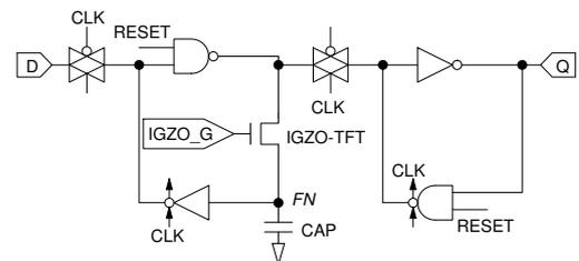
Fig. 1. A series IGZO SR FF architecture without area overhead.
