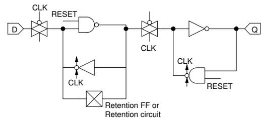
Fig. 2. A parallel IGZO SR FF architecture with area overhead.
