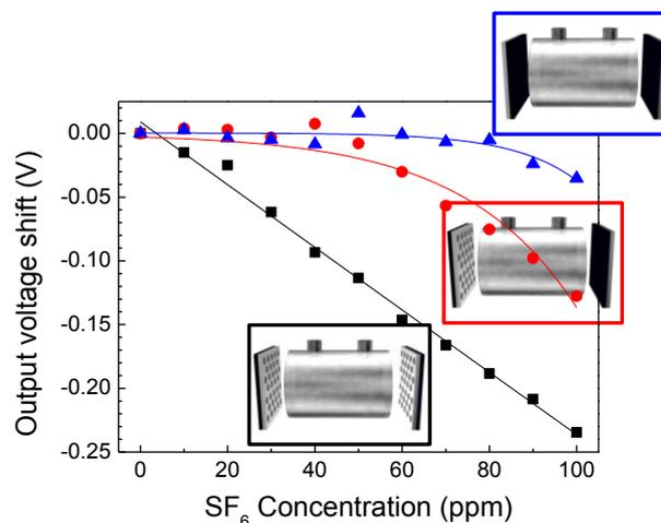
Fig. 1 The response to the SF<sub>6</sub> gas concentration with different three configurations of MHA windows.
