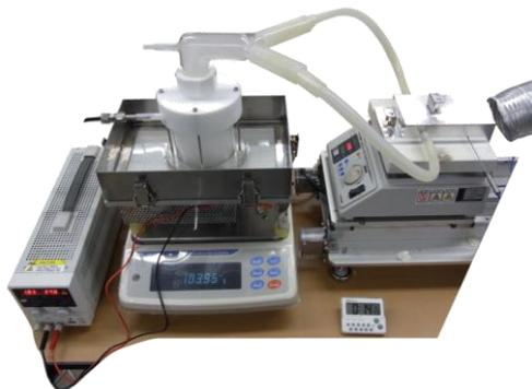
Fig.1 Fine channel type mist CVD system in KUT.
