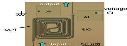
Fig. 2 Optical micrograph of the fabricated MZI (arm length is 5 mm)
