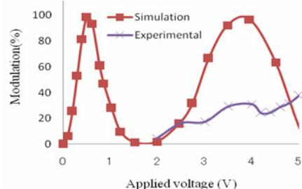
Fig. 3 Modulation versus applied voltage. The length of p and n regions are 0.3 μm and  $N_A=N_D=5.0 \times 10^{18} \text{ cm}^{-3}$ .
