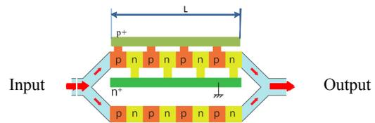
Fig. 1 Structure of Si MZI optical modulator with cascaded p/n junctions
