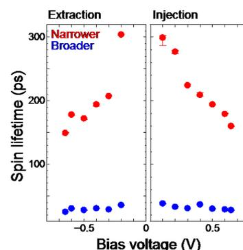
Fig.3 Spin lifetime as a function of bias voltage at 10K for spin injection and extraction measurements.
