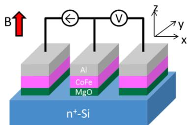
Fig.1 Device structure and measurement setup for three-terminal spin accumulation method.
