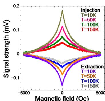
Fig.2 Hanle-effect signals at 10-150K for spin injection and extraction measurements.
