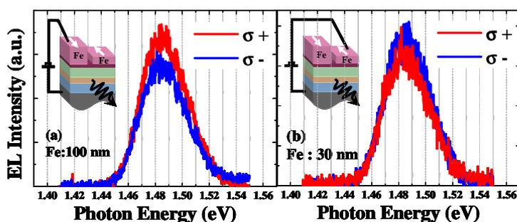
Figs.1  $\sigma^+$  and  $\sigma^-$  EL spectra for samples with flowing a current through with a (a) 100 nm and (b) 30 nm thickness Fe electrode. Magnetization of electrodes is exhibits anti-parallel magnetization configuration.
