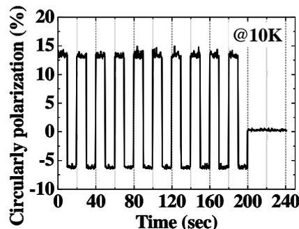
Fig. 2 Experimental data showing electrical helicity switching of circularly polarized light.
