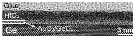
**Fig. 1:** TEM image of O<sub>2</sub> (2.2 nm)/Al<sub>2</sub>O<sub>3</sub> (0.2 nm)/Ge structure with a 500 W PPO for 15 s.
