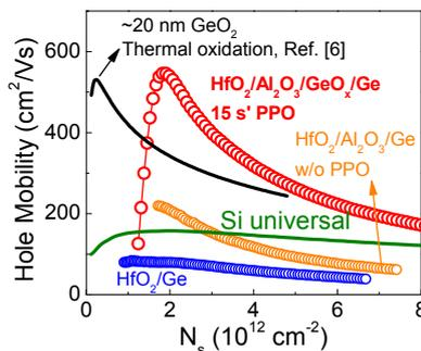
**Fig. 3:** Mobility of Ge pMOSFETs having different MOS interfaces.
