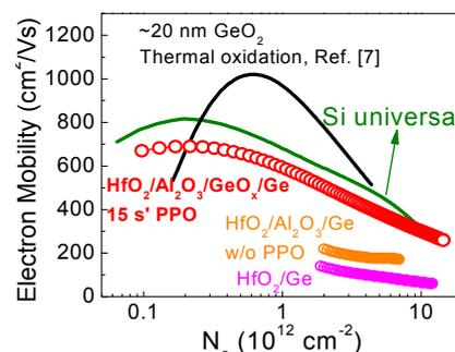
**Fig. 4:** Mobility of Ge nMOSFETs having different MOS interfaces.
