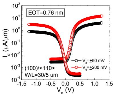
**Fig. 2:**  $I_d$ - $V_g$  curve of the Ge p- and n-MOSFET with the HfO<sub>2</sub>/Al<sub>2</sub>O<sub>3</sub>/GeO<sub>x</sub>/Ge gate stack having 15 s' PPO.
