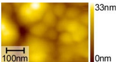
Fig. 1 Topographic image of Si-nanocolumnar structure covered with an ultrathin Au layer.
