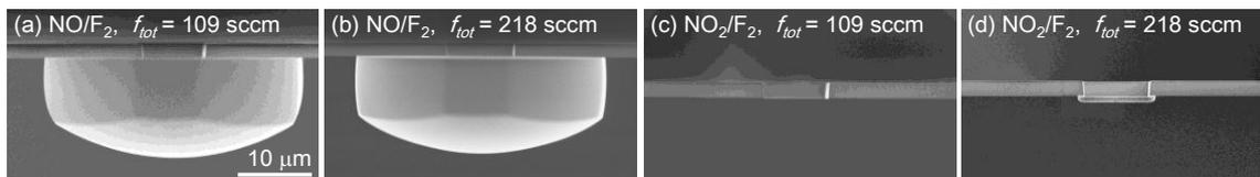
Fig.1 Cross-sectional SEM images after chemical dry etching of Si in Ar/NO/F<sub>2</sub> at total flow rates of (a) 109 sccm (b) and 218 sccm, and in Ar/NO<sub>2</sub>/F<sub>2</sub> at total flow rates of (c) 109 sccm, and (d) 218 sccm. Etching was performed while maintaining the substrate temperature at 300 °C and the pressure at 600 Pa.
