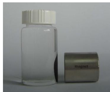
Figure 2 Photographs of Magnetic separation po-MWCNTs/iron oxides solution.
