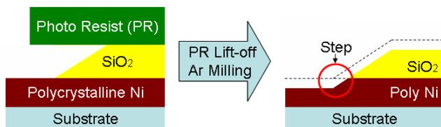
Fig.1 Step-making Process
