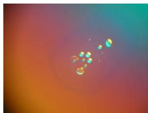
Fig. 2: Damage of external cavity output mirror
