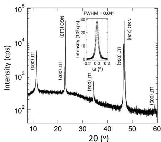
Figure 1 XRD pattern of LLT thin film on NGO (110) substrate. The inset shows rocking curve of LLT (004) with a FWHM of 0.04°.
