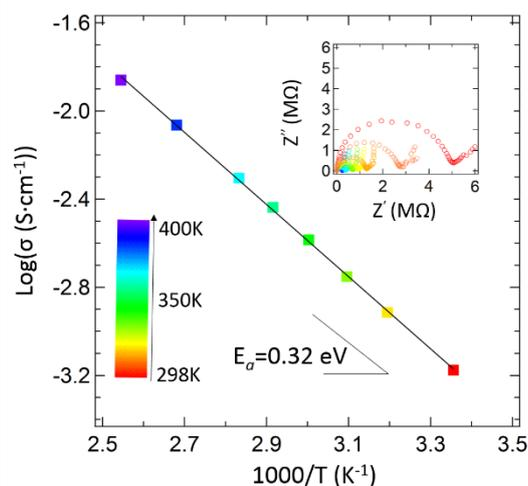
Figure 2 Arrhenius plot of 60 nm thick LLT film on NGO at [1-10] direction. The inset shows complex impedance plots at each temperature.
