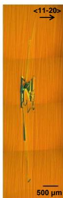
Fig. 1 Microscope image of a stacking fault (3C-inclusion).
