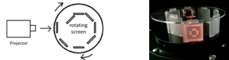
(a)Arrangement of the proposed 3D system (b)Sliced image projection Fig.1 Principle of 3D image formation
