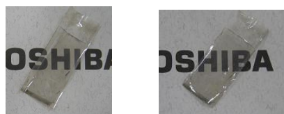
Fig.2 Photograph of h-rGO/AgNW/PMMA film (2cm width, Run 1) before (left) and after (right) \text{NaBH}_4 treatment
