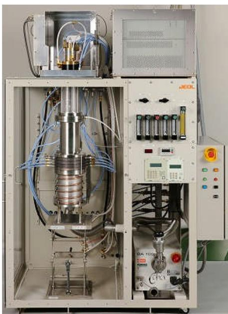
Fig.1 The RF6kW Compact Thermal Plasma System
