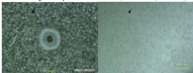
Fig. 2 Microscopic image of ED-B (in Vacuum, 1100°C, 8h, left: ×100, right: ×2000)
