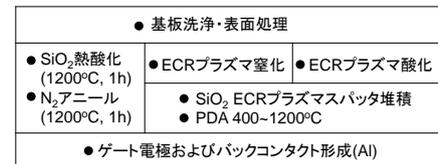
Fig. 1 Procedure of sample preparation for 3C-SiC MOS capacitors.
