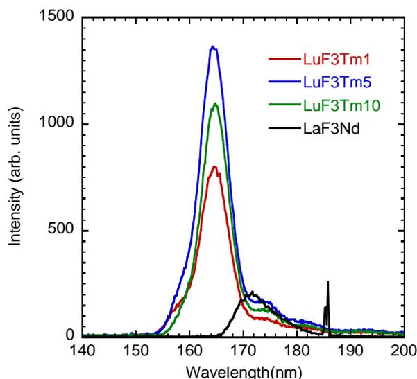
Figure 1. Comparison of X-ray-excited radioluminescence spectra of LuF<sub>3</sub>:Tm samples with that of LaF<sub>3</sub>:Nd 8% reference crystal
