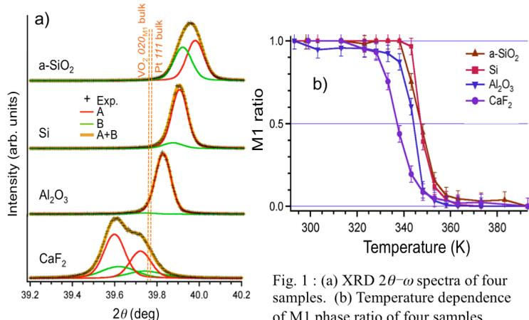
Fig. 1 : (a) XRD  $2\theta$ - $\omega$  spectra of four samples. (b) Temperature dependence of M1 phase ratio of four samples.
