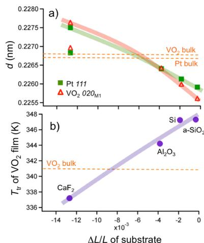
Fig. 2 : (a) Out-of-plane lattice spacings of Pt 111 and VO<sub>2</sub> 020<sub>M1</sub> diffractions, and (b)  $T_{tr}$  of VO<sub>2</sub> films, as functions of  $\Delta L/L$  of the substrates.
