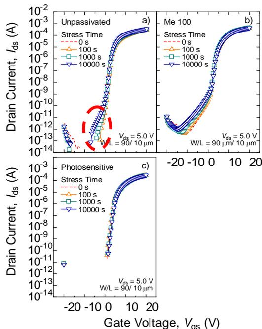
Fig. 1. Variation of transfer characteristics after NBS ( $V_{gs} = -20$ V) for a) unpassivated TFT, b) methylsilsesquioxane passivated TFT, c) photosensitive passivated TFT. Hump effect is highlighted by the red circle.
