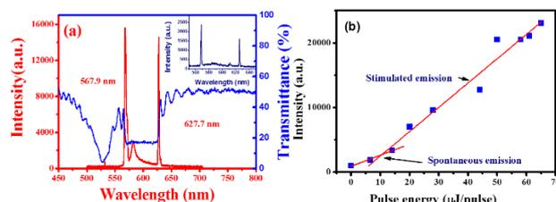
Fig. 2(a) Emission spectra from capillary tube infilling CLC with (red curve) and transmission spectrum of CLC (blue curve). Fig. 2(b) In-out characteristics measured from dye-doped CLCs in capillary tube .
