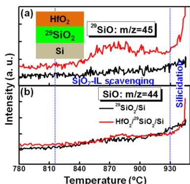
**Fig. 1** TDS results of desorption from HfO<sub>2</sub>/<sup>29</sup>SiO<sub>2</sub>/Si and <sup>29</sup>SiO<sub>2</sub>/Si stacks for (a) m/z=45 and (b) m/z=44.
