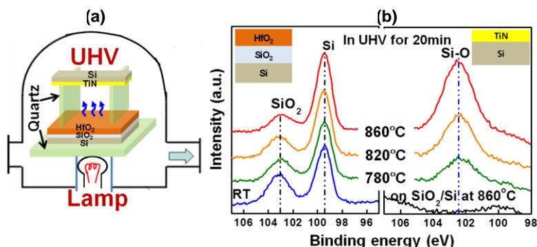
**Fig. 2** (a) Schematics of experiment to collect desorbed species during SiO<sub>2</sub>-IL scavenging in HfO<sub>2</sub>/SiO<sub>2</sub>/Si stack by TiN/Si cap. (b) XPS results (Si2p) of both HfO<sub>2</sub>/SiO<sub>2</sub>/Si stack and TiN/Si cap after UHV-PDA, including the as-grown sample and TiN cap on SiO<sub>2</sub>/Si stack.
